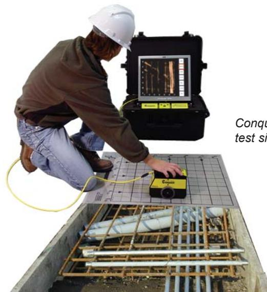
*Conquest on the test sidewalk.*
